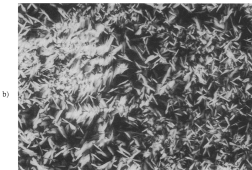
Figure 1: Representative optical polarized micrographs (100x) of the focal conic fan shaped texture displayed by : a) 13(0/100) upon cooling at 5^{\circ}\text{C}/\text{min} from the isotropic phase to 164^{\circ}\text{C} ; b) 13(20/80) upon cooling at 5^{\circ}\text{C}/\text{min} from the isotropic phase to 159^{\circ}\text{C} and annealing for 5 minutes.
